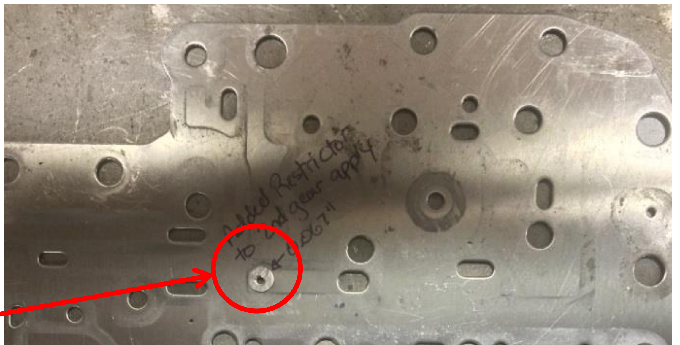
Chamfered to clear the new plug and restrictor
