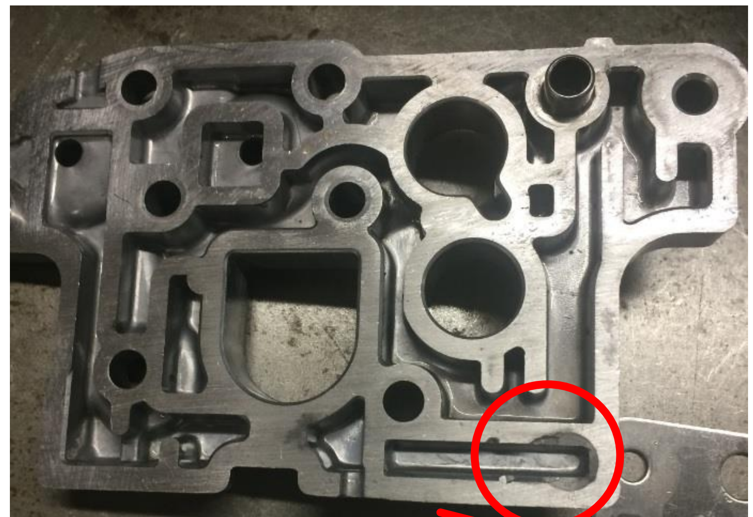
Chamfered to clear the new plug and restrictor
